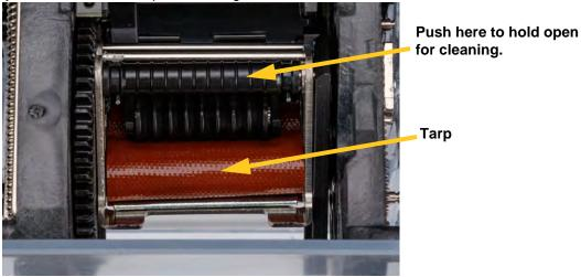
5. Using the moistened swab, clean the tarp. Make sure the tarp is free of dust, debris and label adhesive build-up.
