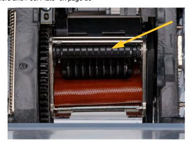
• If using the bulk label roll adapter, the tension may not be correct. Turn the knob on the bulk label roll adapter clockwise to take up slack in the labels. See "Loading Labels on the Bulk Label Roll Adapter" on page 25.
