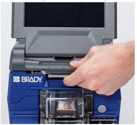
2. To remove the ribbon in the printer, pinch together the tabs on either side of the ribbon cartridge and pull the ribbon cartridge out of the printer.
