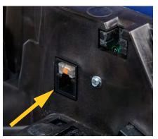
5. Clean the **ribbon out sensor** in the printer chassis with a clean swab dipped in isopropyl alcohol.
