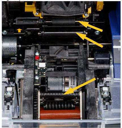
7. Dip a clean swab in isopropyl alcohol and clean the edge of the peel plate.
