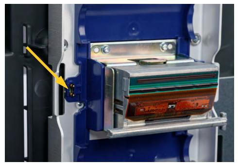
7. Clean the **trigger sensors**, located on either side of the wrapper mechanism with a clean swab dipped in isopropyl alcohol.
