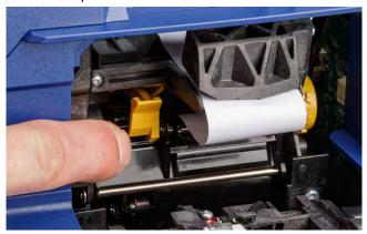
16. Turn the thumbwheel to the right of the peeler to tighten the liner.
