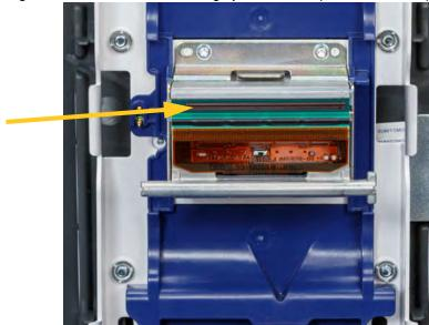
5. Using the moistened swab, thoroughly clean the top surface of the print head.
