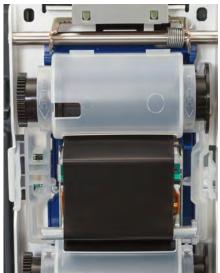
If the ribbon cartridge has been used, turn the top spool to wind used ribbon onto the spool leaving only new, unused ribbon exposed.
